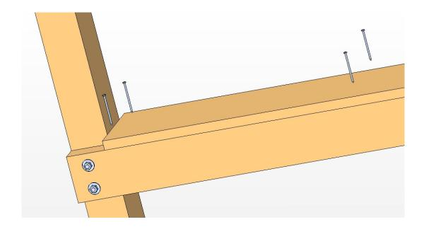
5. Fasten the boards 9 (9\_Lower Slanting Plank) to the boards 6 (6\_Longitudinal Beam) and 7 (7\_Lower Longitudinal Beam) with nails at reciprocal distance 200mm (7,87 inches).
