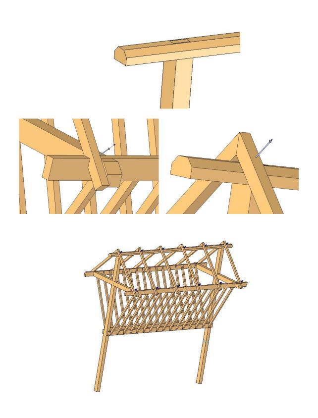
6. Fasten the slats 13 (13\_Distancer) with nails to the edge of the boards 12(12\_Upper Slanting Plank).
