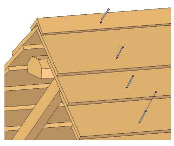
Be careful to use the nails with the same or similar length as given in the Instructions, because the longer nails could stick out through the wood and the animals could get hurt. The details about nailing the construction are given on the next picture
