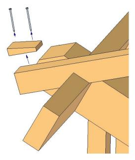
8. The final thing is to fasten the roof boards 14 (14\_Roof Plank) and 15 (15\_Plank With Normal Angle) with nails on top of the construction, and the project is finished.
