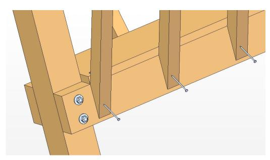
5. Put the beam 10 (10\_Top Longitudinal Beam) on the top and fasten the boards 12 (12\_Upper Slanting Plank) with nails at reciprocal distance 728 mm (28,66 inches)
