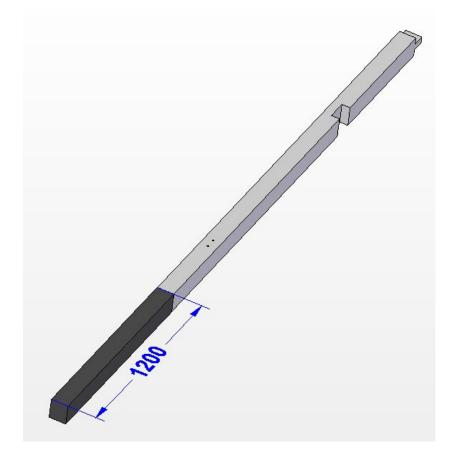
Dig the two holes on depth 1200 mm (47,24 inches) at approximate distance 3640 mm (143,31 inches); then put the pillars into the holes, so that distance is 3640 mm (143,31 inches). Tread the ground around the pillars to make sure the feeder will be stable. If the place on which you plan to put the feeder has loose soil, you should make longer pillars and put it deeper into the ground.
