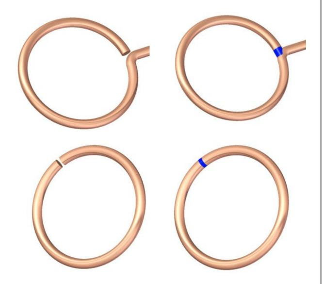
You can use copper or steel wire as a build material. If you choose the copper wire, manufacture will be very easy, but in time some parts will get deformations. So, the best solution is to choose a steel wire, which is not so elastic, but the puzzles will be long lasting.
