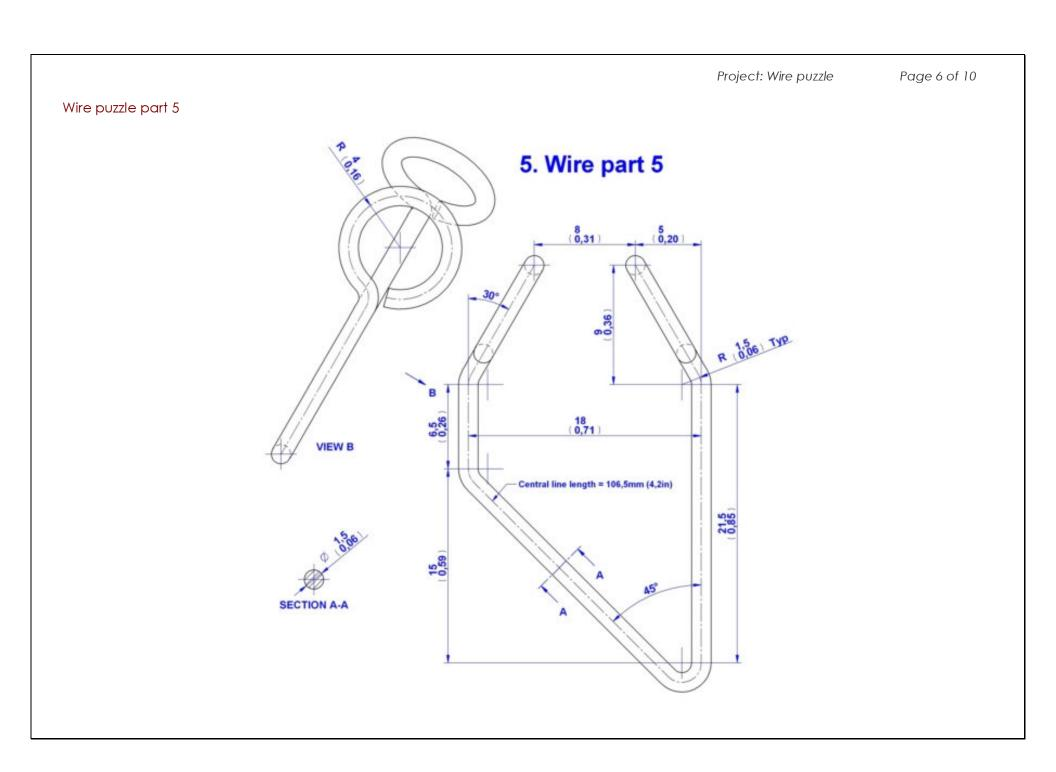
Twist the parts following the documentation. After you twisted it, you can solder the end of wires, as it is shown on pictures, so it wouldn't deform.
